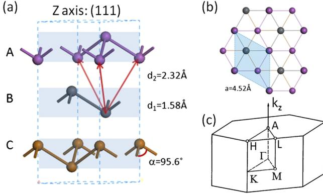
FIG. 1 (color online). (a) The hexagonal unit cell of single-crystal bismuth. (b) The top view of the Bi lattice. (c) The first Brillouin zone of the hexagonal lattice.
