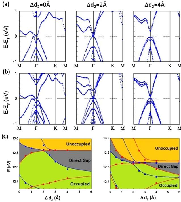
FIG. 2 (color online). The band structure of (a) 2 BLs and (b) 3 BLs under different inter-BL spacing. (c) The energy level at the  $\Gamma$  point of (left) 2 BLs and (right) 3 BLs as a function of the inter-BL spacing. The red (circle) lines indicate even-parity levels. The blue (square) lines indicate odd-parity levels.
