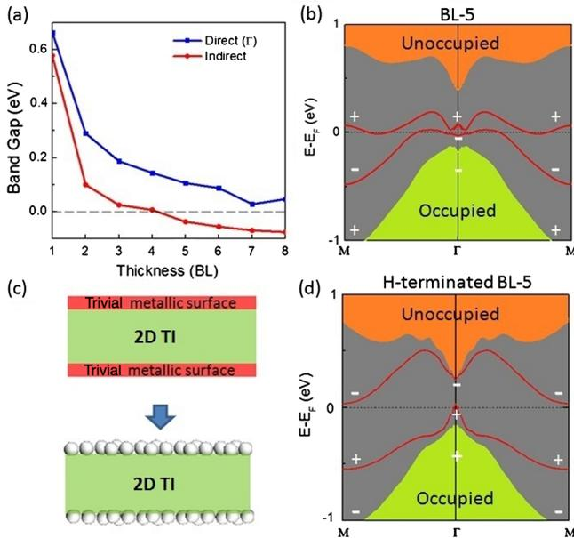
FIG. 3 (color online). (a) The direct ( $\Gamma$  point) and indirect band gap as a function of the film thickness. (b) The band structure and the parity information of 5 BLs. (c) A schematic depiction of the electronic property of a Bi (111) film before and after the H termination. (d) The band structure and the parity information of H-terminated 5 BLs.
